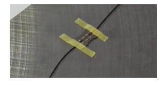
**Spot welding of the sensor to the surface:** The T211 is surrounded by two SS304 metal shells which enable spotwelding the sensor to the monitored structure. There are 8 spot-welds needed to be done in order to properly secure the T211.
