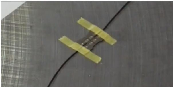
**Spot welding of the sensor to the surface:** The T211 is surrounded by two SS304 metal shells which enable spot-welding the sensor to the monitored structure. There are 8 spot-welds needed to be done in order to properly secure the T211.
