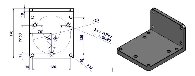
**T510 Tilt Sensor Mounting Plate**
