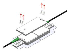
Mount the T220 Pre-Strain Dial Tool to the T220 sensor: Install the 6 parts and 4 screws in the kit as shown below:
